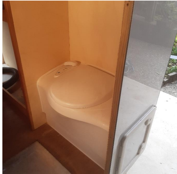
Example of NZMCA member fitting a 'fixed' toilet into a slide on camper vehicle. This camper is still under construction, however the toilet will be behind folding doors in its own compartment.
