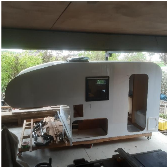
Example of NZMCA member fitting a 'fixed' toilet into a slide on camper vehicle. This camper is still under construction, however the toilet will be behind folding doors in its own compartment.
