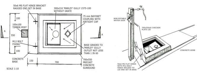
Figure 2 - DUAL VEHICLE DUMP POINT IN ACCORDANCE WITH NZS 5465:2001
