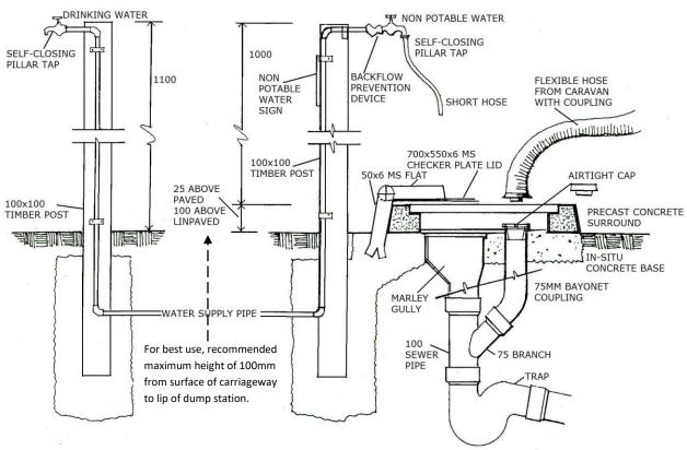
If fresh water tap/s are to be included in the installation, it is recommended that they be installed as far away from the D/S carriageway as the site will allow. With the increasing numbers using the facilities congestion can occur frequently.
